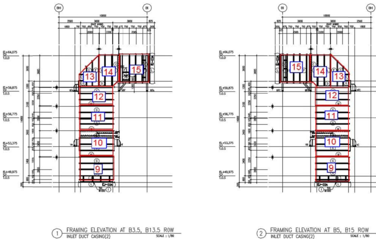
Figure 6.6 Site Assembly Parts of Inlet Duct (No.9 ~ 15)
