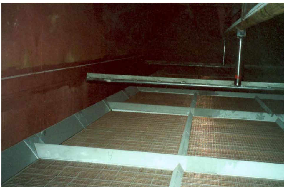
Fig. 14 Dust hoods on top of the modules
