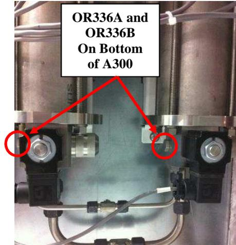
**Figure 30 – Drain Orifice Locations**
