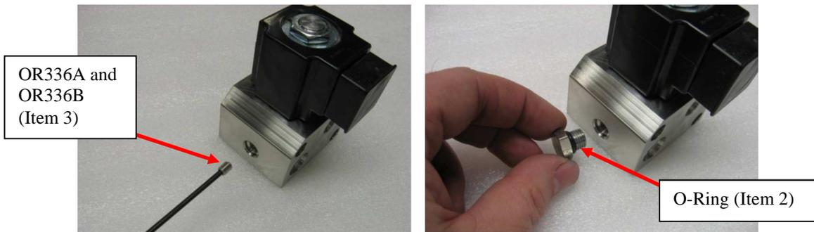
**Figure 31 – Drain Orifice Replacement**
