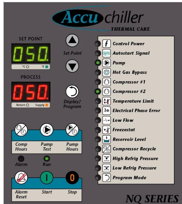
The chiller includes a controller to perform all control functions directly from the front panel. When Control Power is applied, the controller initiates a diagnostic test of each indicating light and display segments by briefly lighting each sequentially. As part of this initial diagnostic test, the program revision level displays for a moment. After the initial diagnostic sequence is completed, the controller is ready for operation.
