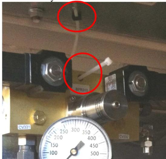
**Figure 33 - Cable Tie Connection**
