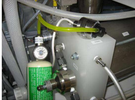
**Figure 11 - Calibration Gas for CG220**
