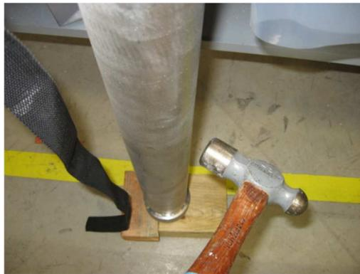
**Figure 46 - Desiccant at the Top of the Cylinder and Tapping the Cylinder**
