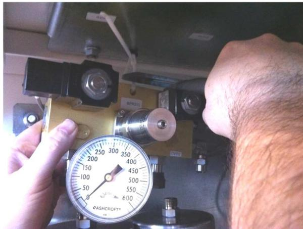
**Figure 49 - Upper Manifold Block**
