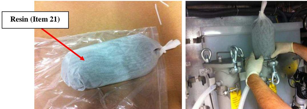
Figure 26 - Guard Bed Filter DI Bag
