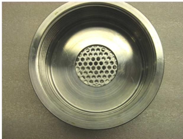
**Figure 39 – Cap with Screen Support**
