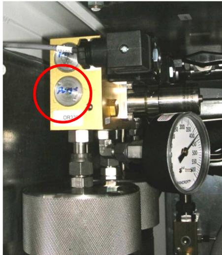
**Figure 50 – Orifice Cap**
