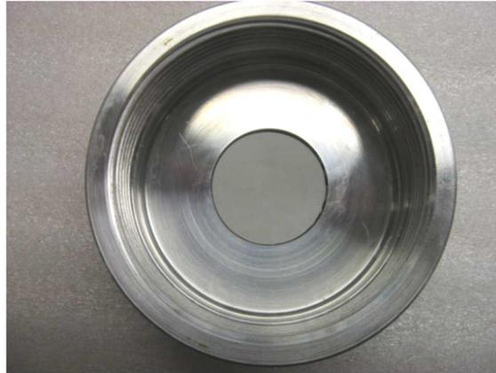
**Figure 40 – Cap with Filter Screen**
