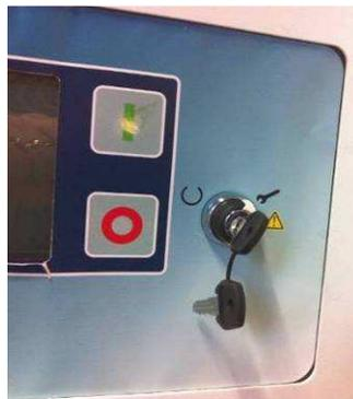
Figure 9 - Key in Service Bypass Mode
